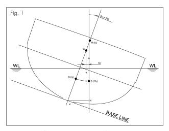
Position of the various centers of an inclined hull.
