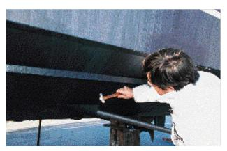
The surveyor uses a hammer to sound the hull shell and assess its condition.
