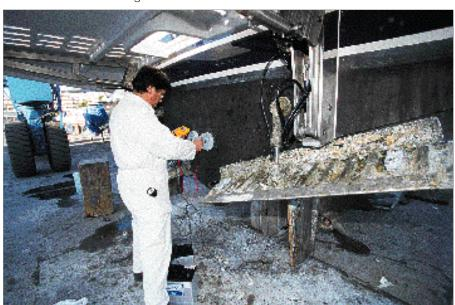
Checking the connections of the sacrificial anodes.
