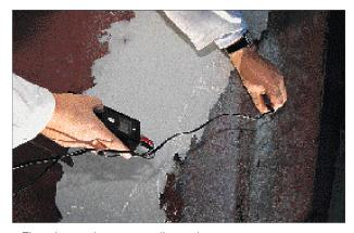
The ultrasonic gauge allows the surveyor to measure the thickness of the aluminum and steel hull plating.
