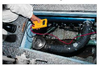
A voltmeter is used by the surveyor to check the efficiency of the bonding system and a reference cell.
