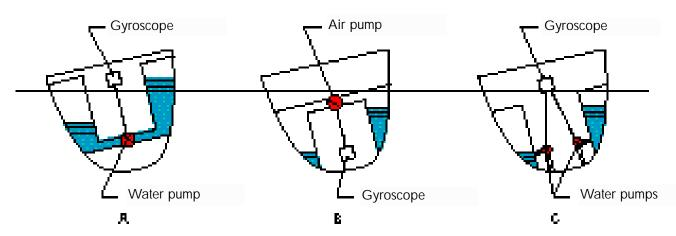
Three types of anti-roll tanks of the active type, with a roll sensor, water and air pumps.
