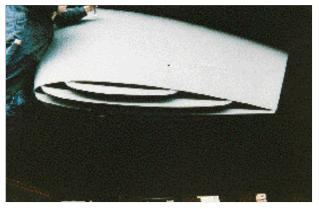
Section of a high speed stabilizer fin.
