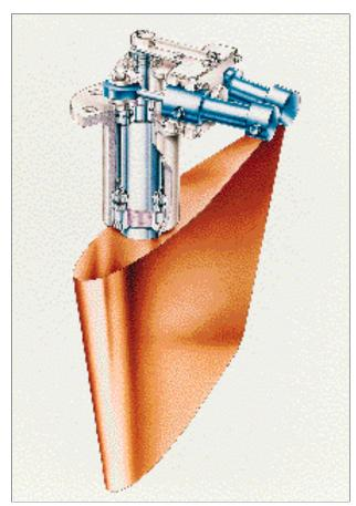
can be found in a well known reference book, "Theory of Wing Sections", which should be part of every yacht designer's library. The most currently used section for stabilizers and rudders is known as NACA 0015. It has a maximum thickness equal to 15% of the
