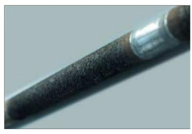
This propeller shaft suffered from DC stray currrent corrosion.
