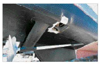
The role of a strut is to support the shaft forward of the propeller. Therefore its shape is very important.
