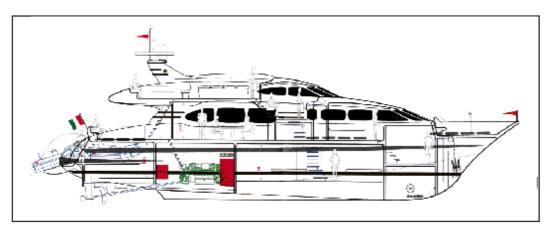
A direct line installation moves the engine and the center of gravity forward.
