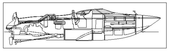
The V-drive allows the installation of the engine further aft while preserving the advantages of a conventional driveline.
