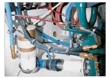
The stuffing box must not be leaking and is to be frequently monitored.
