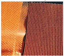
Honeycomb can be used on tight curved surfaces.
