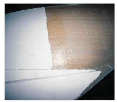
On a female molds, gel coat becomes the last layer.
