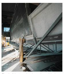
The hull bottom laminate is molded on a male mold while the topsides have fabricated on temporary female molds.
