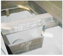
Intregral tanks can be built in composites hulls.
