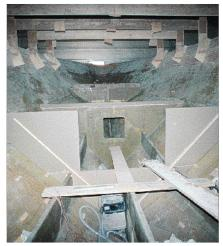
Foam cored sandwich bulkheads improve both sound and thermal insulations.
